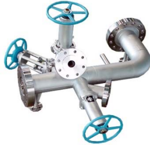
900psi-8"/5" Jacketed Y-Globe valve with 2 x 3" Drain valves
