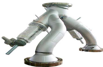
W3Z type 3-way Isolation Valve 150psi-34"/28"x 28"/24" Flange connection Jacketed, Electric Motor operated
