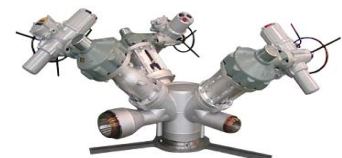
W4S type 160K-12"/8" x 10"/7"x 6"/4" BW Jacketed 4-way Valve Electric motor operation (control valve)
